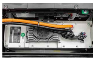
(Option) Lithium battery with the on-board charger (48V, 20A) (Excluding model F2)
